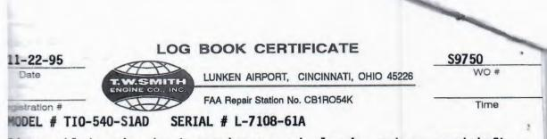
Disassembled engine due to crankcase crack, leaving rods on crankshaft. Washed all parts with solvent. Assembled engine with new camshaft, main bearings, gaskets and regrind lifter bodies. Honed all cylinders for ring finish, cleaned pistons and installed new rings. All other parts of the engine were reused and are in serviceable condition. This engine assembled according to parts manual and current regulations. This engine is in serviceable condition and is ready for return to service. End.
