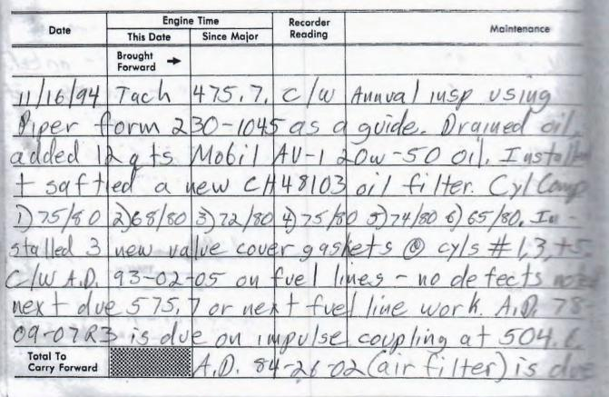
Signature Certificate No. and Remarks 580.0. Engine runup OKE no fue orail eaks noted. Date 11/10/94 Tach: 475, Total Time 1925, 7 TSMOH 387,7 I certify that this engine has been inspected Shoreline Aviation, Inc. in accordance with an QUNUAL Inspection and Marshfield Municipal -1. MA 02050 617 837-8521 was determined to be in airworthy condition. Sign Edward A Moven 1 A & P# 23445 8337A
