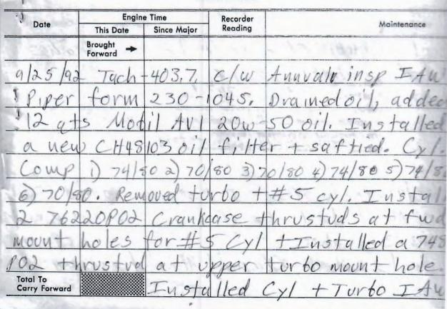
and Remarks Signature Certificate No. Service Manuals. Installed a new exhaust How at wastegate outlet over xhaus pe. c/wAD 92-12-16 AW A.D. - No defects nota due ILLP.S 503.7 or next annual or whenever mes ave disturbed. AD 78 -09-07R3 impulse Coupling) is due at 504. 6 ir filter) is due at 580.0. Wa. runup O KENO fuel or
